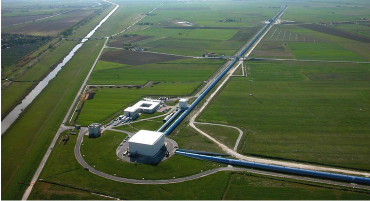
Figure 1: The aerial view of Virgo gravitational wave detector located near Pisa in Italy. The armlength of Michelson interferometer is 3 km. [Image credit: Virgo]
